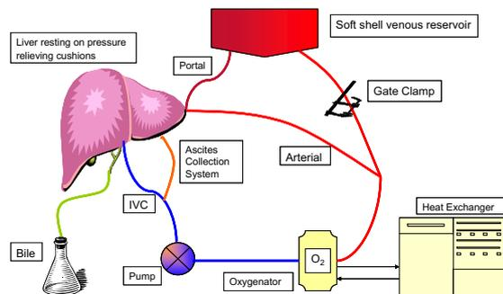
Figure: Schematic Diagram of Perfusion Circuit used in the experiments
