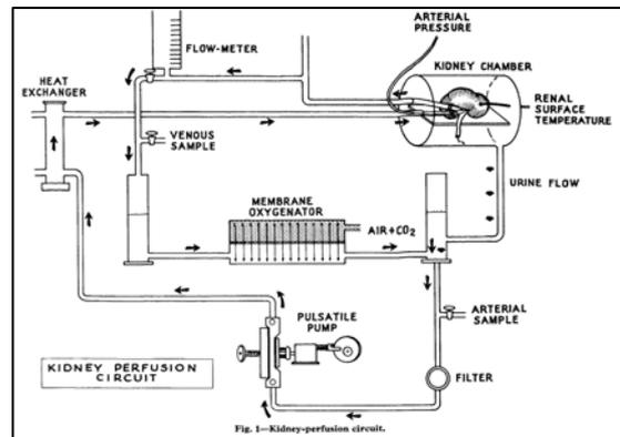
The perfusion circuit used by Belzer for machine perfusion of renal grafts. The current perfusion machines continue to have a broadly similar layout.
